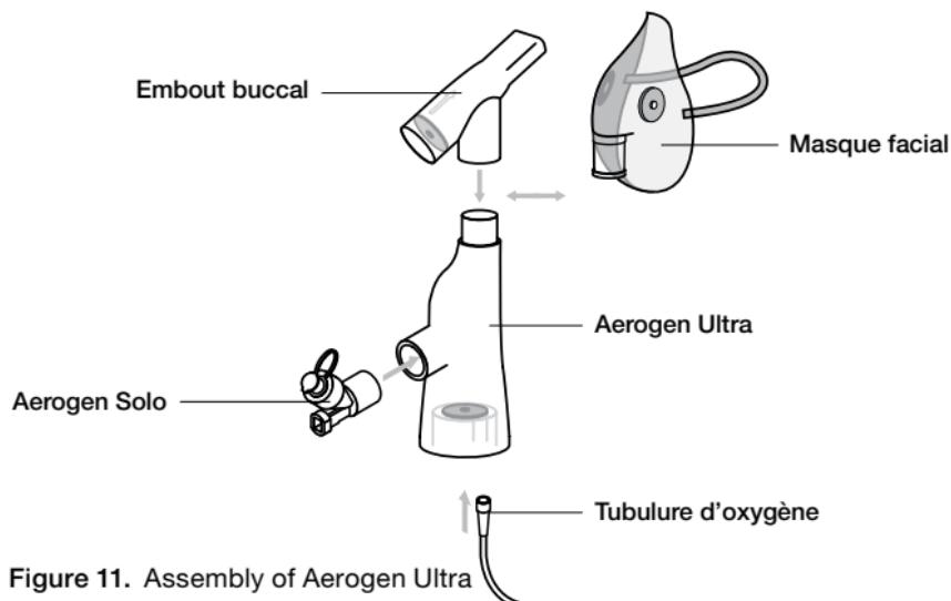
Figure 11. Assembly of Aerogen Ultra
